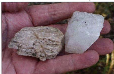
Figure 4. This was the original reason for the Ytterby Mine—high quality feldspar (left) and quartz (right) used in the porcelain industry. Feldspar (taken from German for “Feldspat,” meaning “field spar”) is a general term for alkali and alkaline earth aluminosilicates and is the most common mineral in the earth’s crust, comprising 60 percent. Quartz ( \text{SiO}_2 ) is the second most common mineral. Today the Ytterby area is still littered with large amounts of both minerals.
