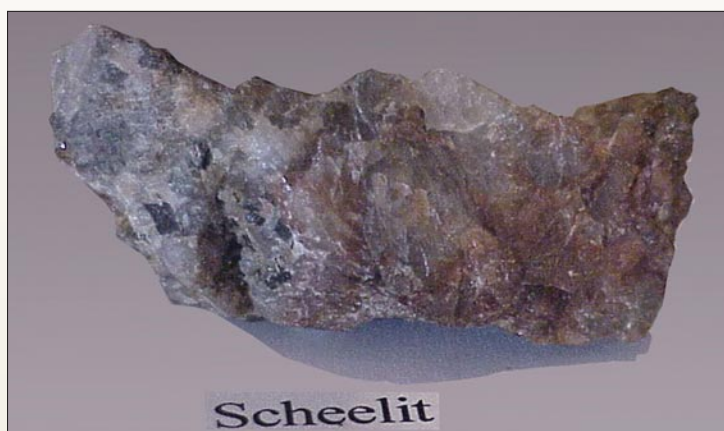
Figure 15. Scheelite (discovered by Cronstedt) sometimes forms octahedral crystals, but it is more commonly amorphous like this specimen. This sample is displayed in the acclaimed Scheele museum in Köping, Sweden. 4c Swedish miners and mineralogists call this form of scheelite “fruset snor” (“frozen snot”) for obvious reasons. 4a Night rock hunters search for this mineral with portable UV lamps, which cause scheelite to fluoresce a beautiful blue, very much like diamond’s fluorescence.
