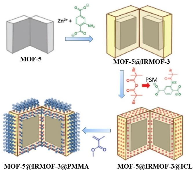
Figure 21. Diagrammatic sketch for the preparation of MOF-5@IRMOF-3@PMMA. Adapted with permission from RSC. [93]
