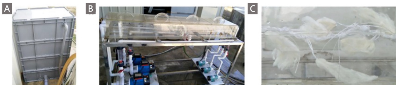
Fig. 42 Recovery of uranium from natural seawater. (A) Seawater reservoir. (B) Adsorption flume. (C) H-ABP fibrous adsorbent immersed in the flume at the beginning of adsorption. Reproduced with permission. 132 Copyright 2019, Royal Society of Chemistry.
