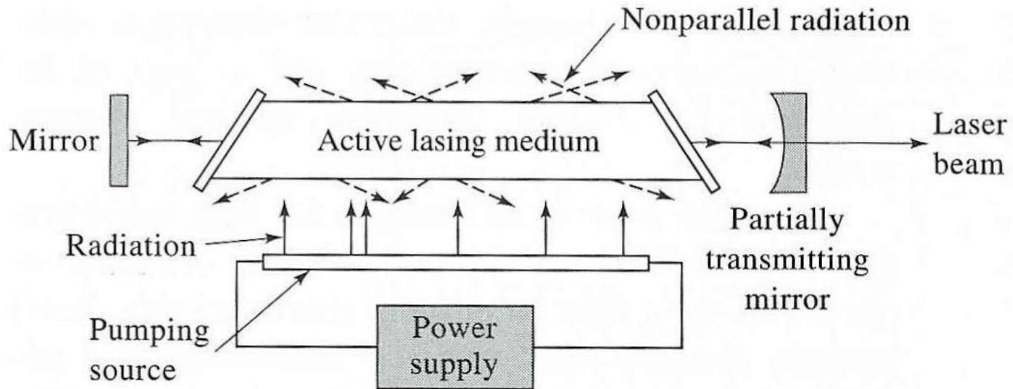
Nonparallel radiation dissipates out the top and bottom of the medium and parallel or coherent radiation is left.
