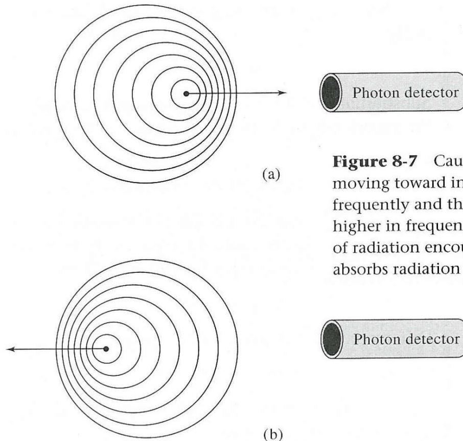
**Figure 8-7** Cause of Doppler broadening. (a) Atom moving toward incoming radiation sees wave crests more frequently and thus absorbs radiation that is actually higher in frequency. (b) Atom moving with the direction of radiation encounters wave crests less often and thus absorbs radiation that is actually of lower frequency.
