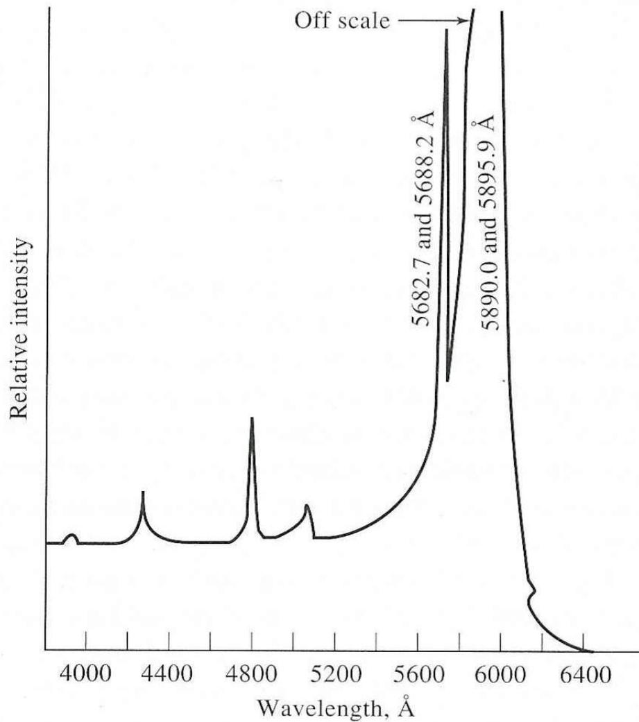
**Figure 8-4** A portion of the flame emission spectrum for sodium.
