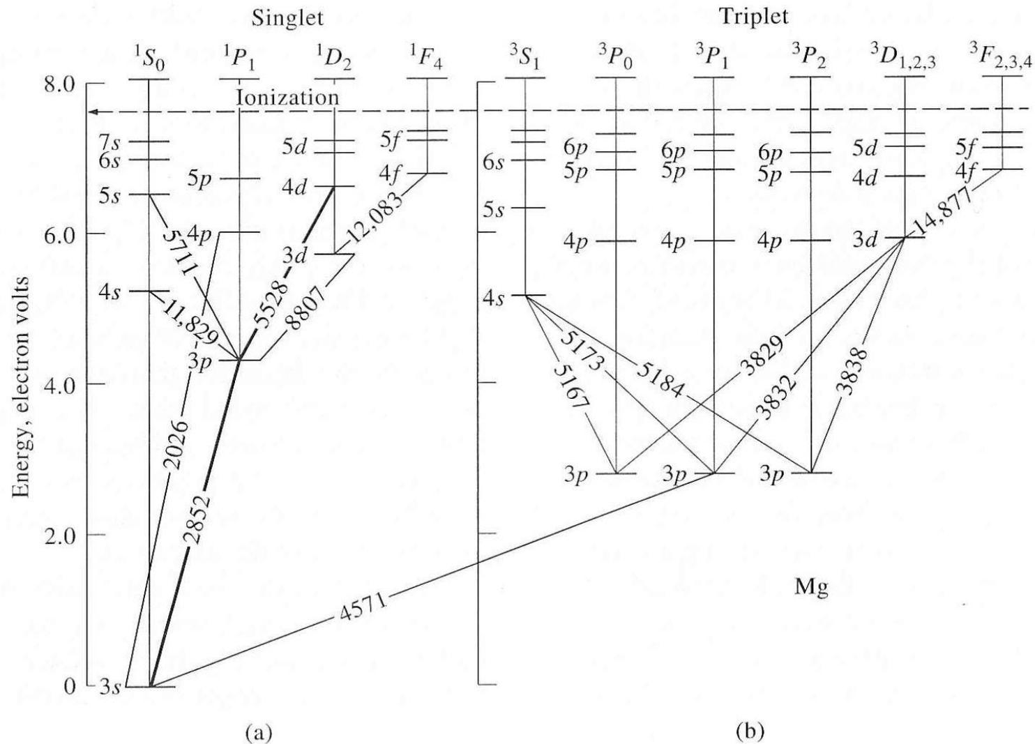
**Figure 8-2** Energy level diagram for atomic magnesium. The relative line intensities are indicated very approximately by the width of the lines between states. Note that a singlet/triplet transition is considerably less probable than a singlet to singlet transition.
