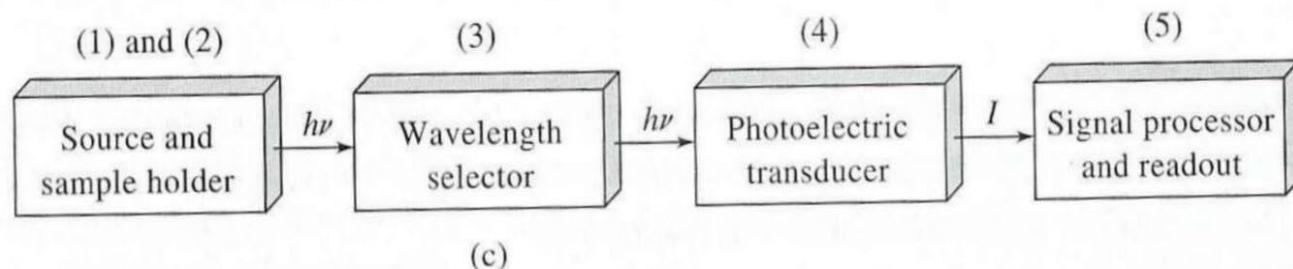
**Figure 7-1** Components of various types of instruments for optical spectroscopy: (a) absorption; (b) fluorescence, phosphorescence, and scattering; (c) emission and chemiluminescence.
