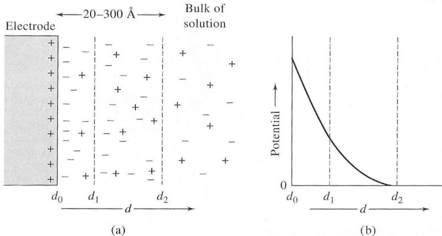
**Figure 22-2** Electrical double layer formed at electrode surface as a result of an applied potential.
