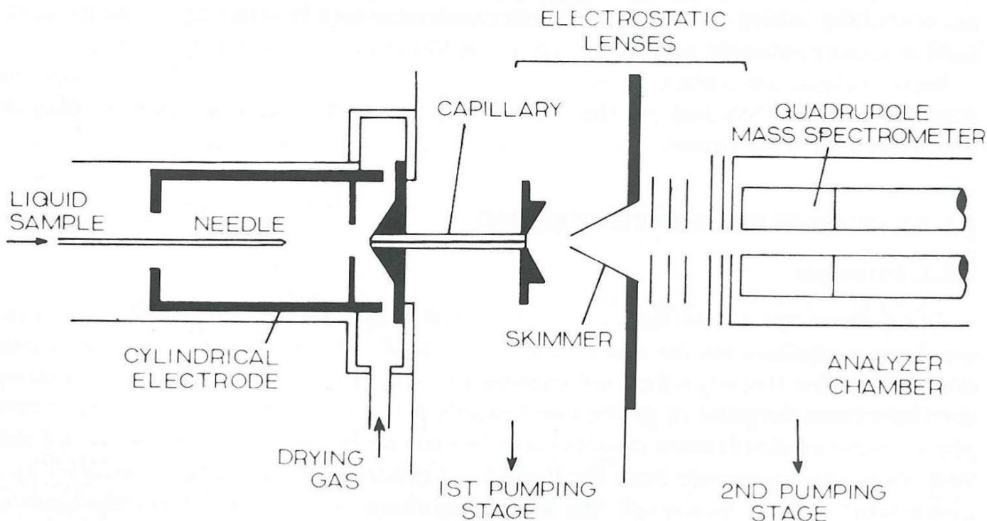
Fig. 1.13. Schematic diagram of the first-generation electrospray LC-MS interface as described by Whitehouse et al. [216]. Reproduced from Ref. [216] with permission. © 1985, American Chemical Society.
