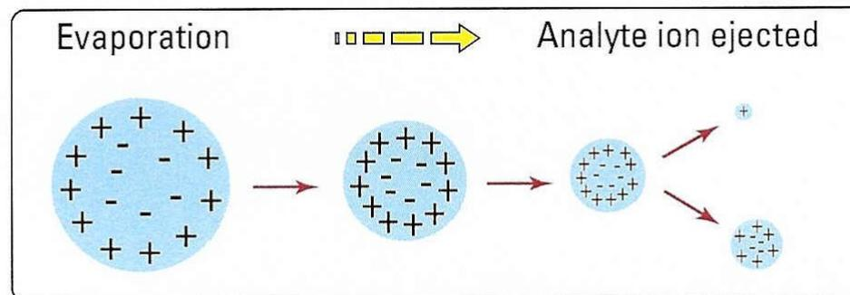
Figure 5. Desorption of ions from solution
