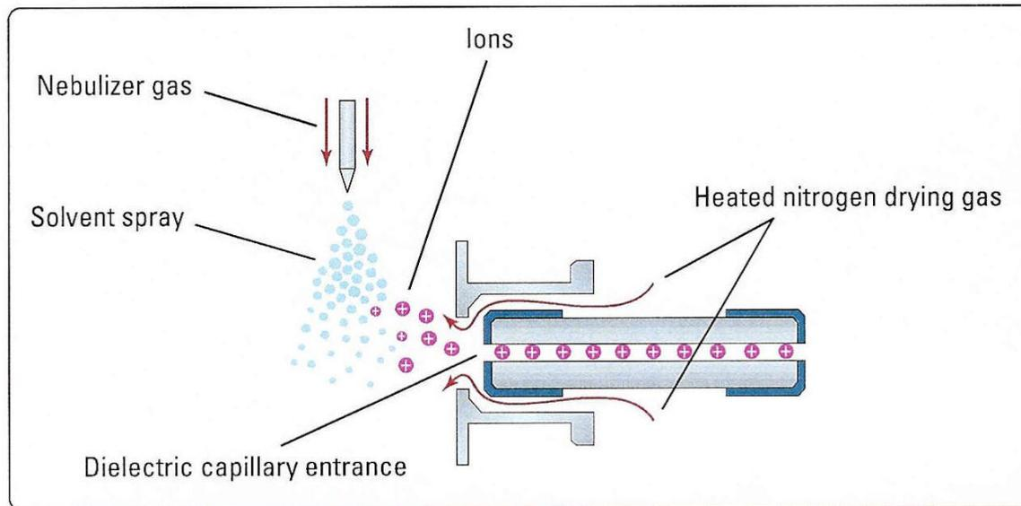
Figure 4. Electrospray ion source
