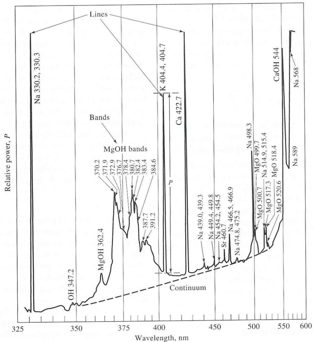
**Figure 6-15** Emission spectrum of a brine obtained with an oxyhydrogen flame.
