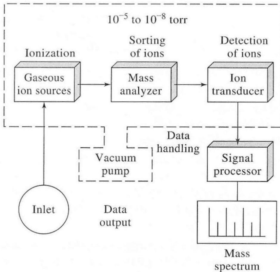
**Figure 11-1** Components of a mass spectrometer.
