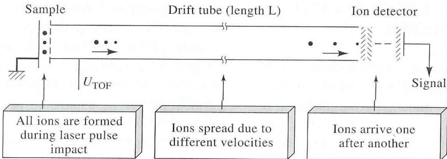
**Figure 11-8** Principle of a time-of-flight mass spectrometer. A bunch of ions produced by a laser probe is accelerated into the drift tube where separation occurs. (From A. H. Verbueken, F. J. Bruynseels, R. Van Grieken, and F. Adams, in *Inorganic Mass Spectrometry*, p. 186. F. Adams, R. Gijbels, and R. Van Grieken, Eds. New York: Wiley, 1988. With permission.)
