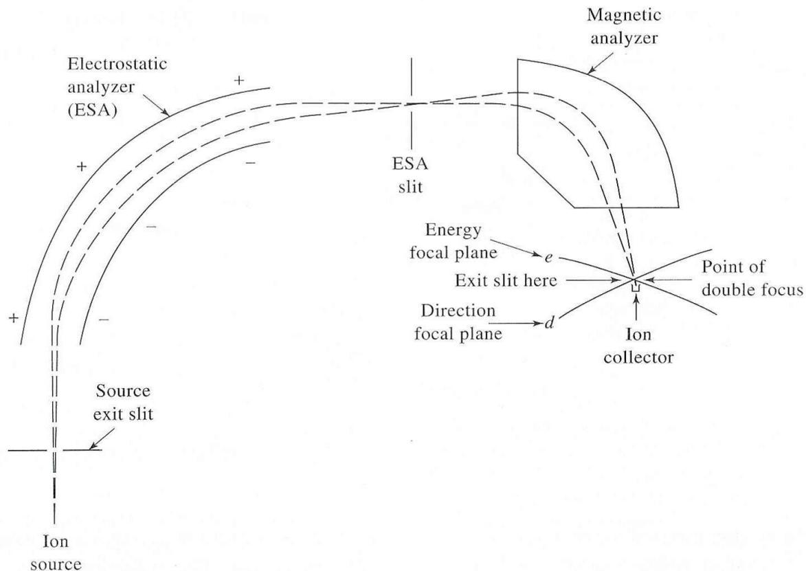
**Figure 20-13** Nier-Johnson design of a double-focusing mass spectrometer.
