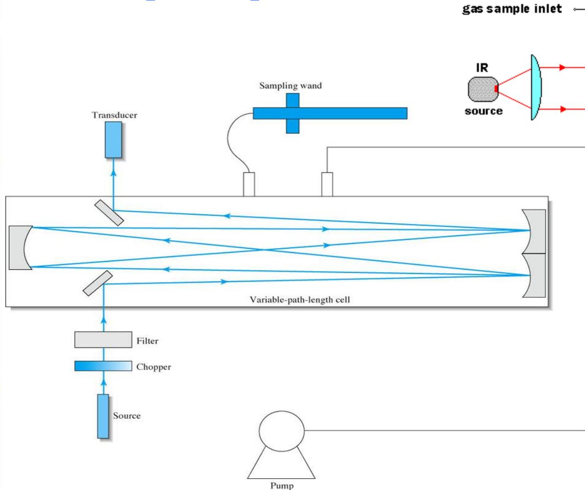
Typical Infrared Photometer
