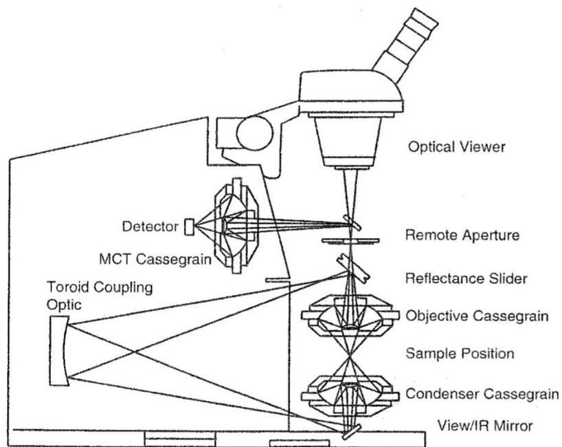
**Figure 4.24** IR microscope schematic with the detector integrated into the microscope. The microscope is usually coupled to a light port on the side of the FTIR spectrometer. The FTIR spectrometer supplies a modulated, collimated beam of light to the microscope. Courtesy of PerkinElmer Instruments, Shelton, CT ([www.perkinelmer.com](http://www.perkinelmer.com)). (From Coates, used with permission.)
