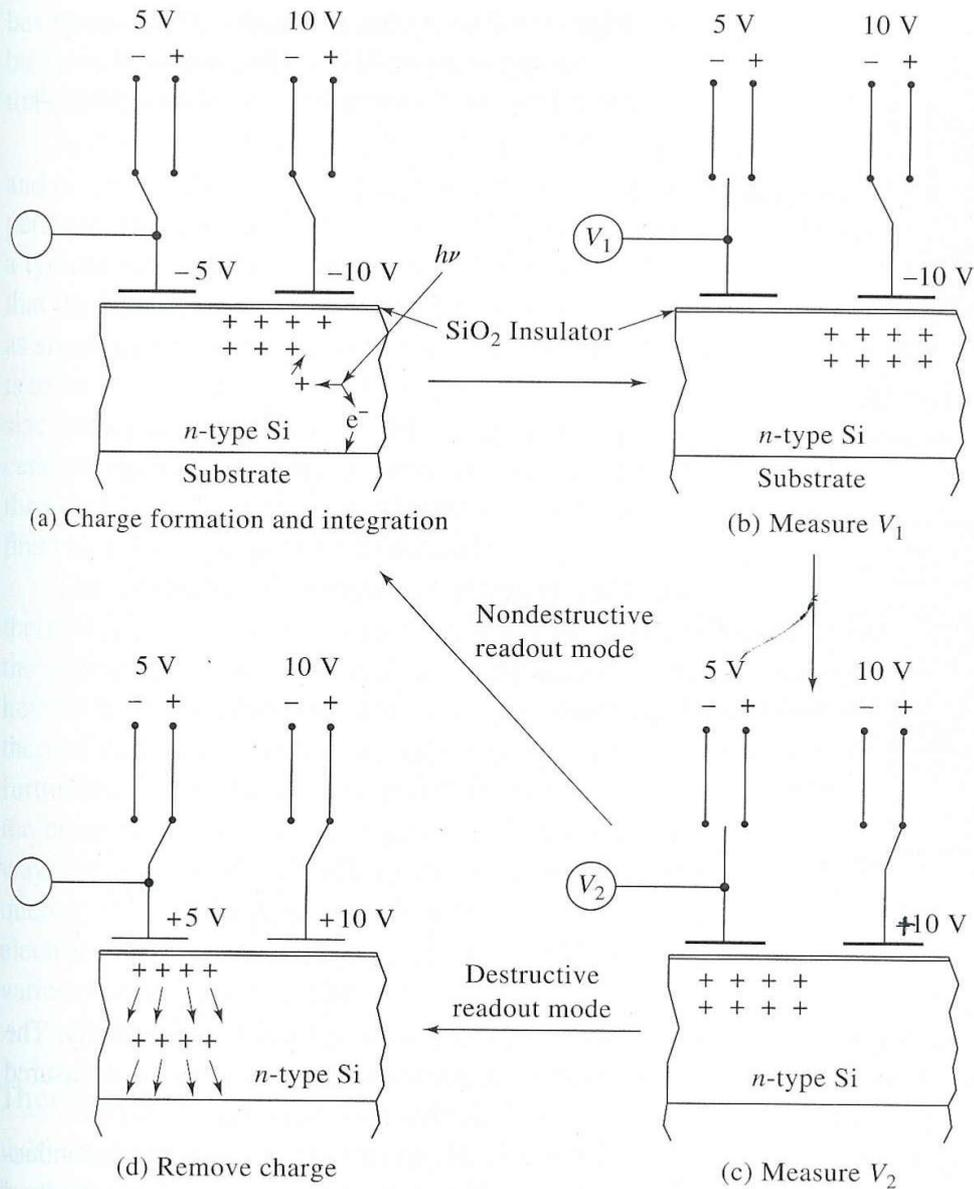
**Figure 7-34** Duty cycle of a charge-injection device: (a) production and storage of charge, (b) first charge measurement, (c) second charge measurement after charge transfer, (d) reinjection of charge into the semiconductor.
