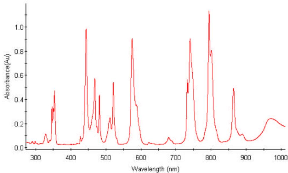
The spectrum of didymium solution: S-3150, SCINCO, measuring time 1 sec.
