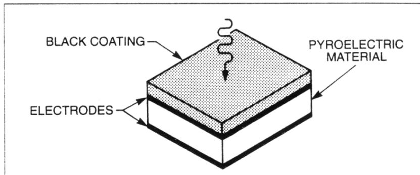
Fig. 6 Schematic of a pyroelectric detector.
