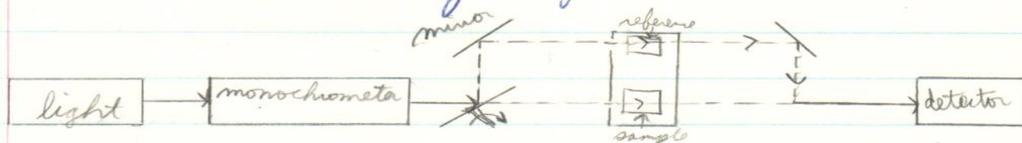
Figure 2: A scanning double-beam spectrometer with dual source, single grating.
