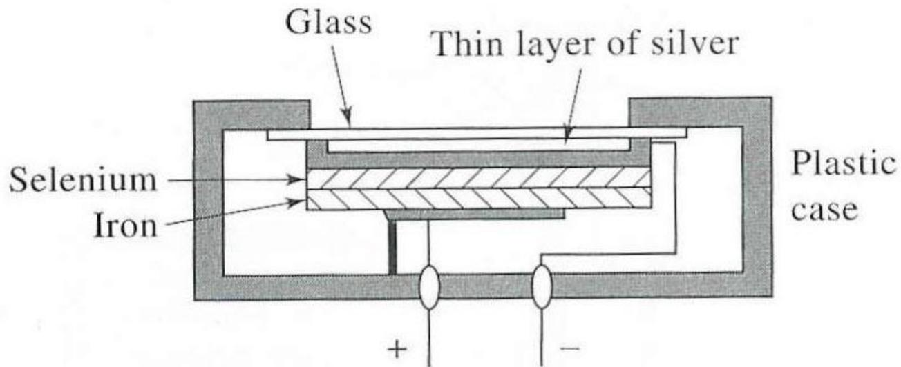
**Figure 7-26** Schematic of a typical barrier-layer cell.
