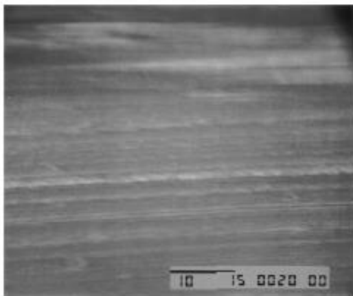
FIGURE 8: Cross-sectional SEM of a CeO 2 /MMT nanocomposite electrodeposited film using potentiostatic conditions at E = 1.10 V and 25°C (bar represents 10 μm).
