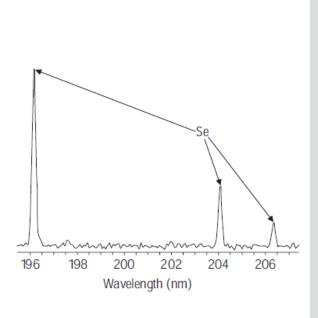
An extract of garlic shows low-level sulfur and selenium compounds important in flavor and nutritional analyses. Selenium is confirmed by its three characteristic atomic lines from 196 to 206 nm.
