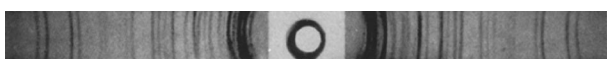
Figure 5. Debye-Scherrer diffraction pattern of solid \alpha -nitrogen at the boiling point of liquid hydrogen (21 K), recorded by Vegard in 1929 with an iron anti-cathode. [35]
