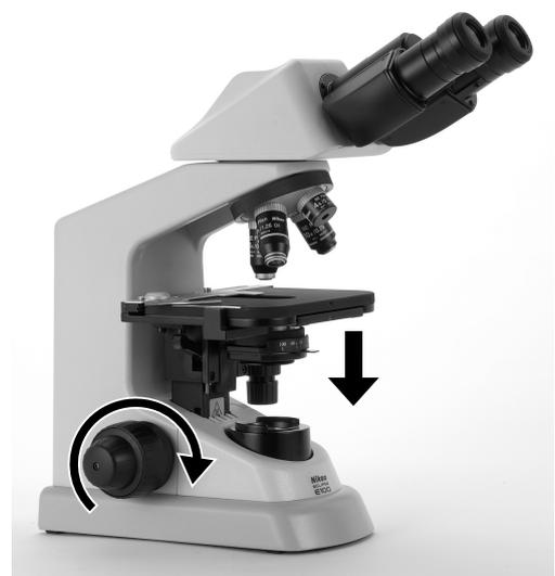
Turn the focus knob as shown to move the stage down.
