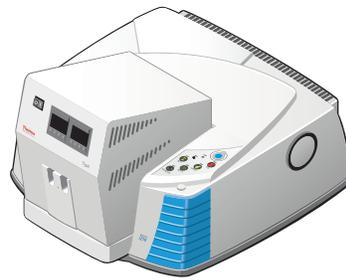
Provides a second sampling area for routine analysis with an accessory and for installing and using large, dedicated accessories like the TGA interface.
