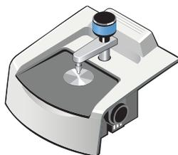
Place the sample on the crystal and apply pressure. A good first sample might be a credit card, an old CD, or a piece of plastic. For liquids, no pressure is needed.
