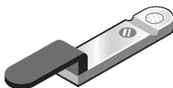
Fill the cup with a sample. A good first sample is a ground aspirin tablet diluted to 3-5% in KBr powder. You do not need to overfill the cup.
