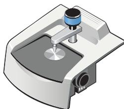
Make sure the pressure device, if included, is not in contact with the crystal. Clean the crystal with a soft cloth and, if needed, an appropriate solvent.
