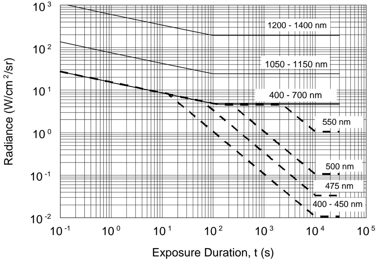
**Figure E-10. Extended source ocular radiance maximum permissible exposures ( 110 milliradian) for visible and near infrared (400 nanometers to 1400 nanometers) (Solid lines are maximum permissible exposures based on thermal effects, and dashed lines are maximum permissible exposures based on photochemical effects)**
