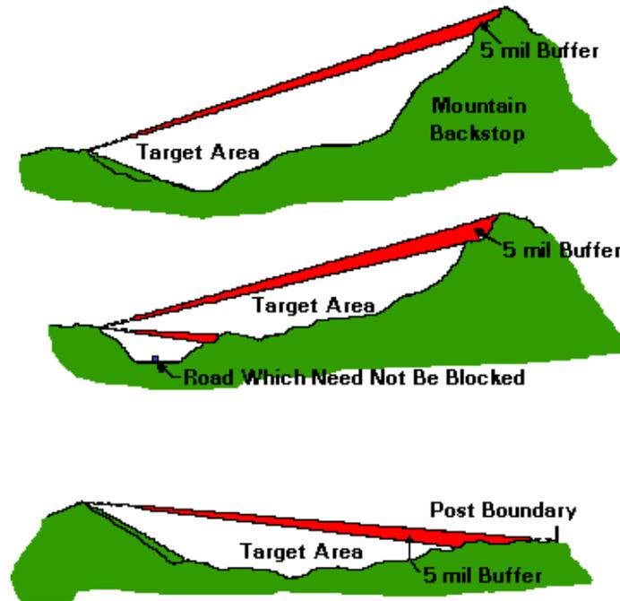
*Figure 6-1. Laser range terrain profiles with backstop*
