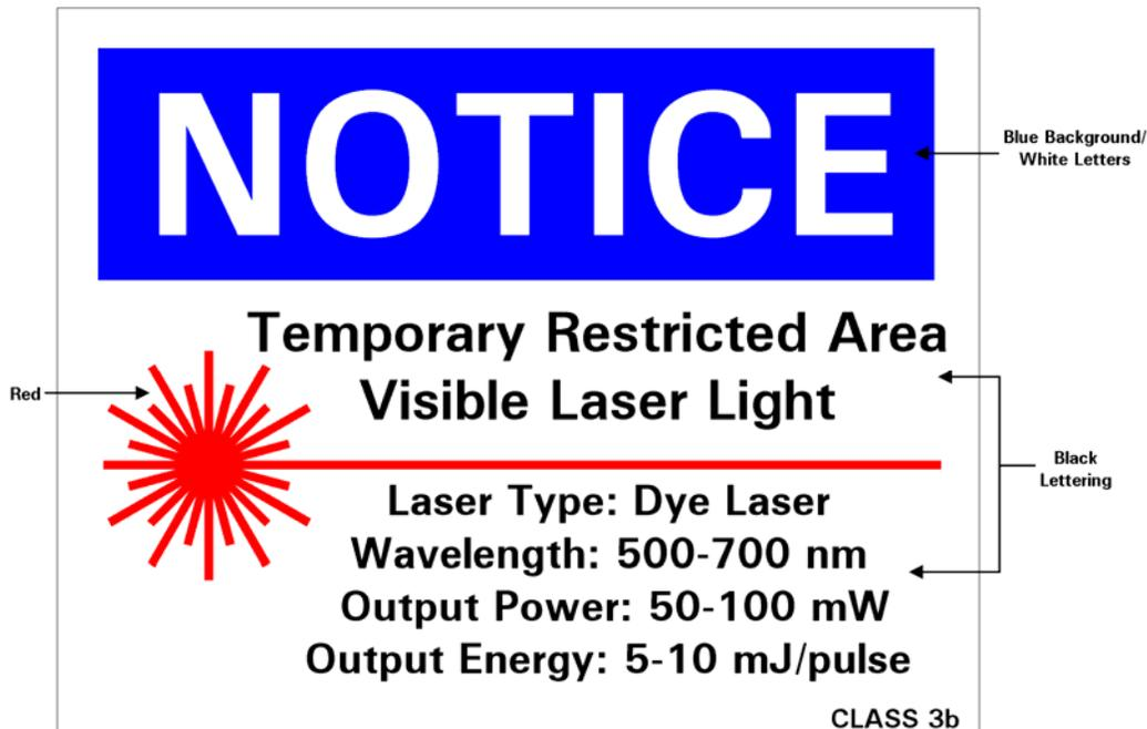
*Figure 5–7. Sample warning sign for temporary laser controlled area*
