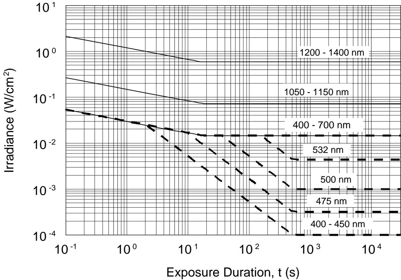
*Figure E-8. Extended source ocular maximum permissible exposures ( = 25 milliradian) for visible and near infrared (400 nanometers to 1400 nanometers) (Solid lines are maximum permissible exposures based on thermal effects, and dashed lines are maximum permissible exposures based on photochemical effects)*
