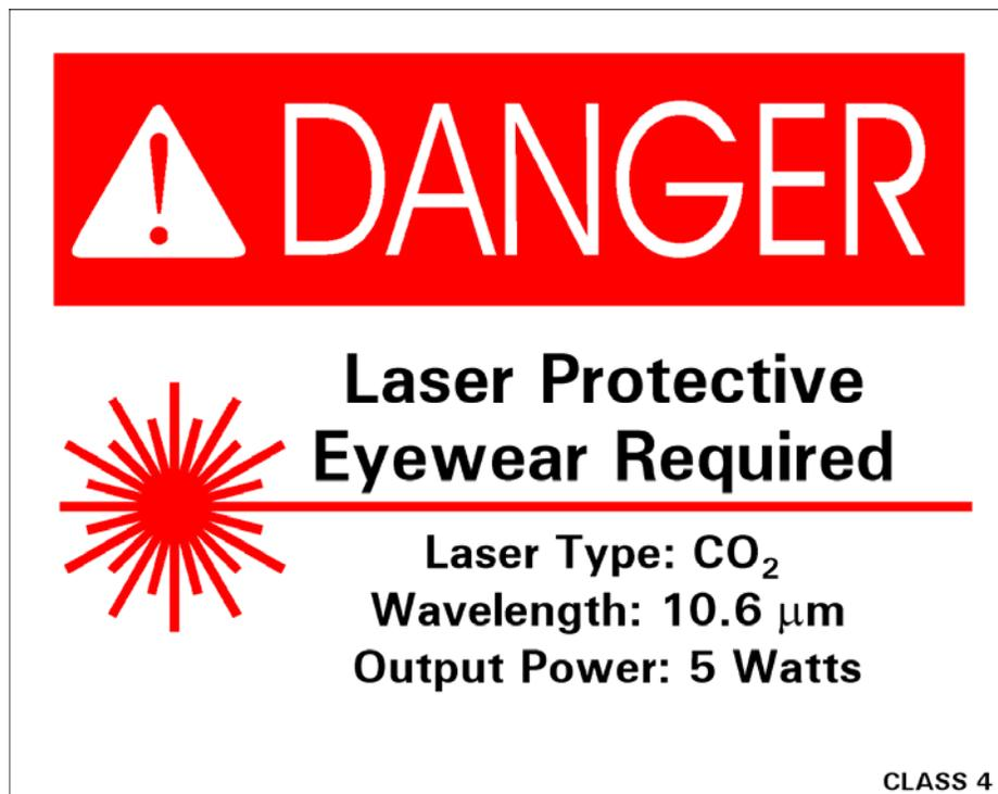
*Figure 5–5. Sample warning sign for Class 4 carbon dioxide laser*
