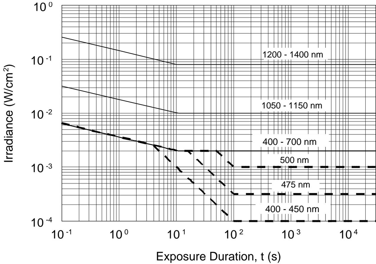
*Figure E-6. Extended source ocular maximum permissible exposures ( = 3 milliradian) for visible and near infrared (400 nanometers to 1400 nanometers) (Solid lines are maximum permissible exposures based on thermal effects, and dashed lines are maximum permissible exposures based on photochemical effects)*
