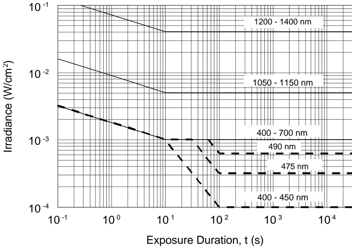
*Figure E-5. Small source ocular maximum permissible exposures ( 1.5 milliradian) for visible and near infrared (400 nanometers to 1400 nanometers) (Solid lines are maximum permissible exposures based on thermal effects, and dashed lines are maximum permissible exposures based on photochemical effects)*
