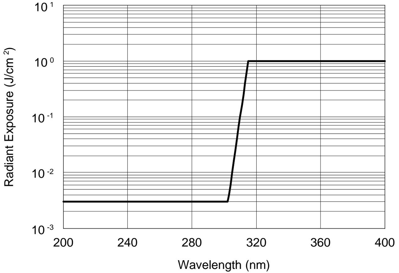
*Figure E-2. Maximum permissible exposures for small and extended source ultraviolet radiation for exposure durations from 10<sup>-9</sup> to 30,000 seconds for ocular exposures and 10<sup>-9</sup> to 10<sup>3</sup> seconds for skin exposure*
