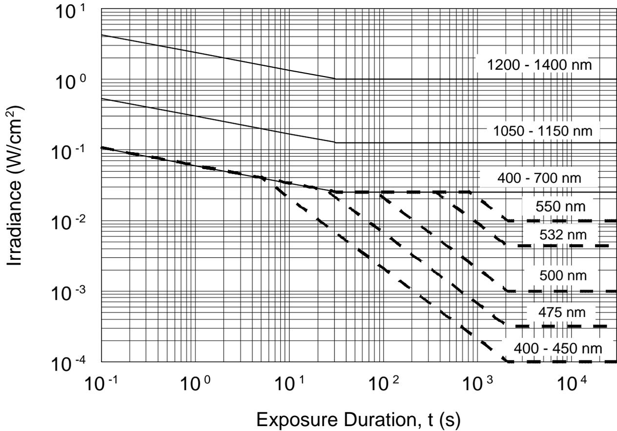
*Figure E-9. Extended source ocular maximum permissible exposures ( = 50 milliradian) for visible and near infrared (400 nanometers to 1400 nanometers) (Solid lines are maximum permissible exposures based on thermal effects, and dashed lines are maximum permissible exposures based on photochemical effects)*
