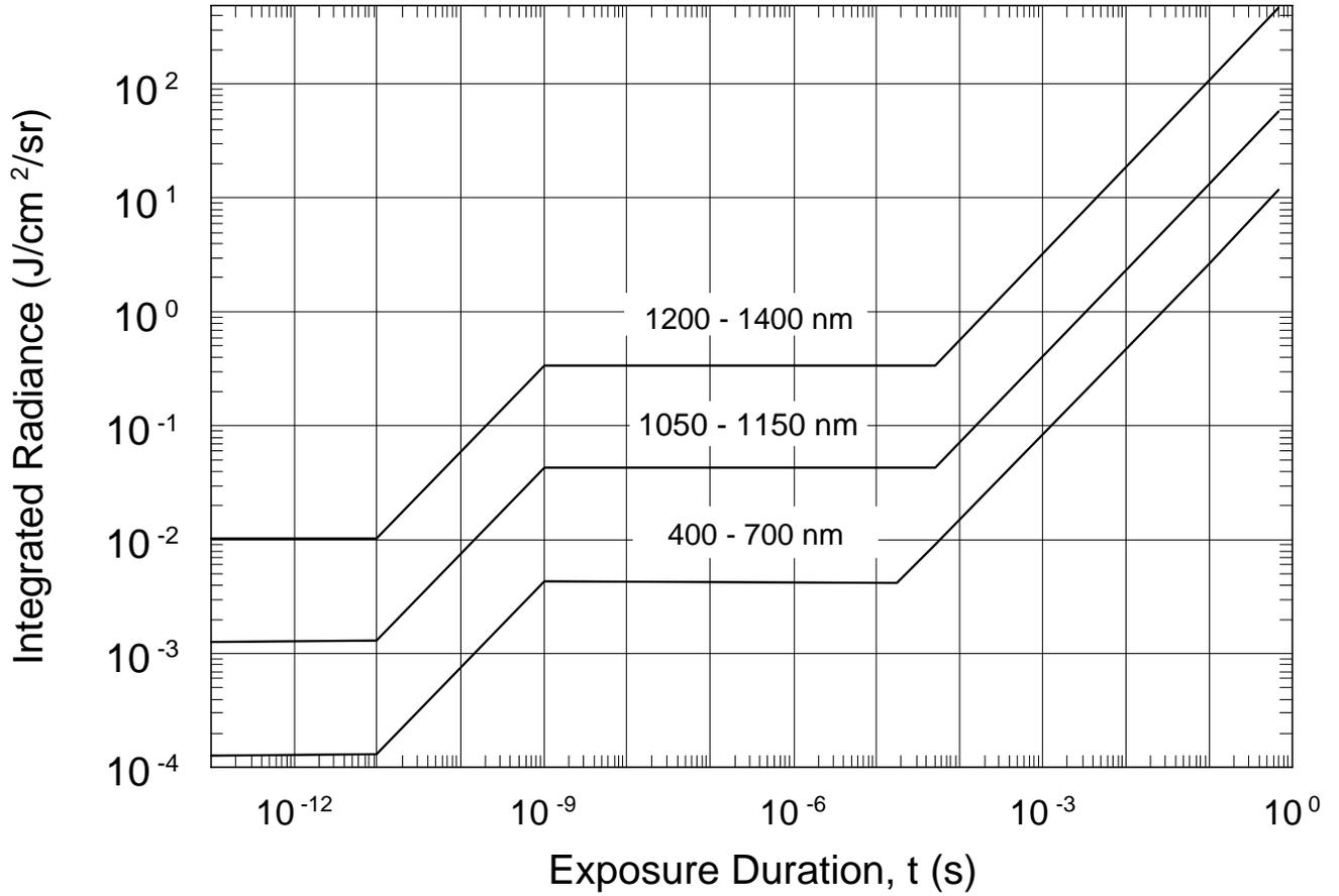
*Figure E-11. Extended source ocular radiance maximum permissible exposures ( 100 milliradian) for visible and near infrared (400 nanometers to 1400 nanometers) for pulsed or continuous wave exposures less than 1 second*
