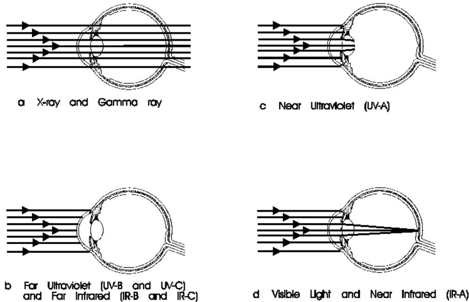
**Figure 3–3. Absorption of electromagnetic radiation by the eye**
