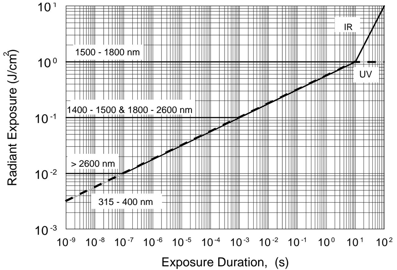
*Figure E-3. Maximum permissible exposures for ultraviolet (315 nanometers to 400 nanometers) and infrared (1400 nanometers to 1 millimeter) for single pulses or continuous exposure to small or extended sources*
