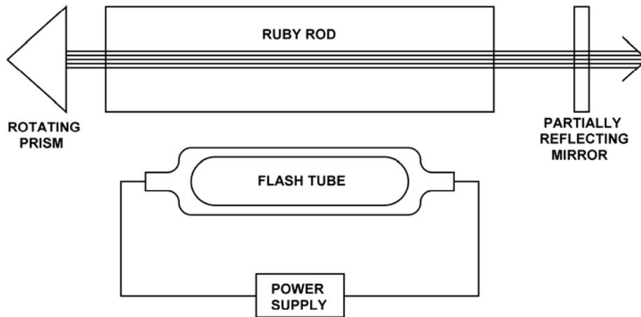
*Figure 2-6. Schematic of solid-state laser with optical pumping*
