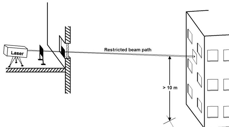
Note: The test range is established by limiting beam elevation and azimuth to ensure that the beam strikes a diffuse backstop; the beam path is above occupied areas
