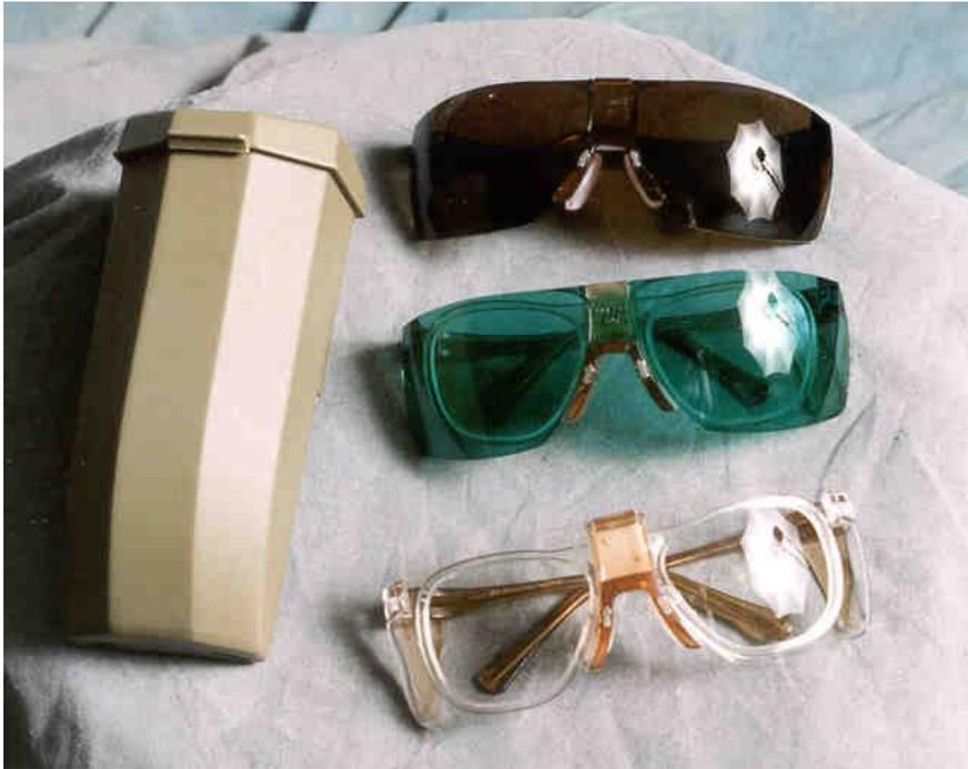
**Figure 7-4. Ballistic and laser protective spectacles**
