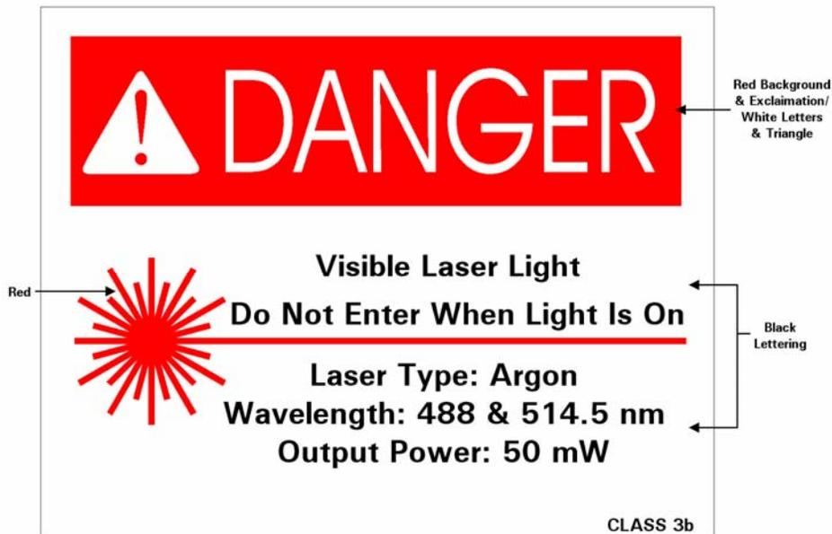
Figure 5-1. Sample warning sign for Class 3b laser
