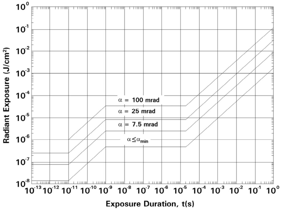
*Figure E-4. Maximum permissible exposures for ocular exposure to visible laser radiation (400 nanometers to 700 nanometers) for single pulses or continuous exposure (small or extended sources)*
