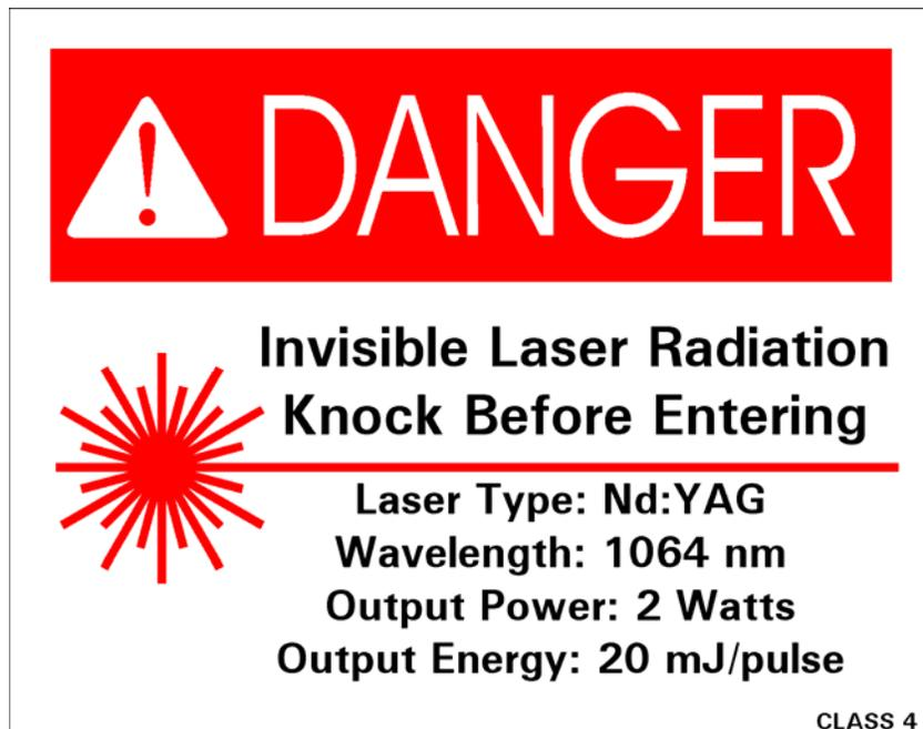
Figure 5-2. Sample warning sign for Class 4 laser
