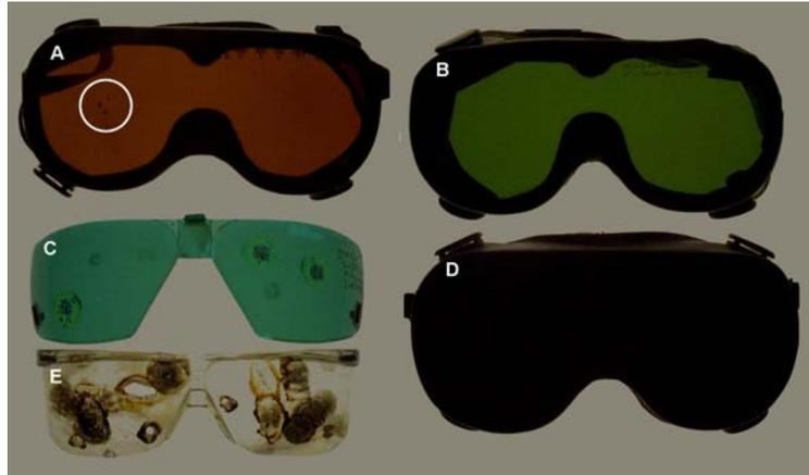
**Figure 7–3. Examples of damage to laser protective devices**
