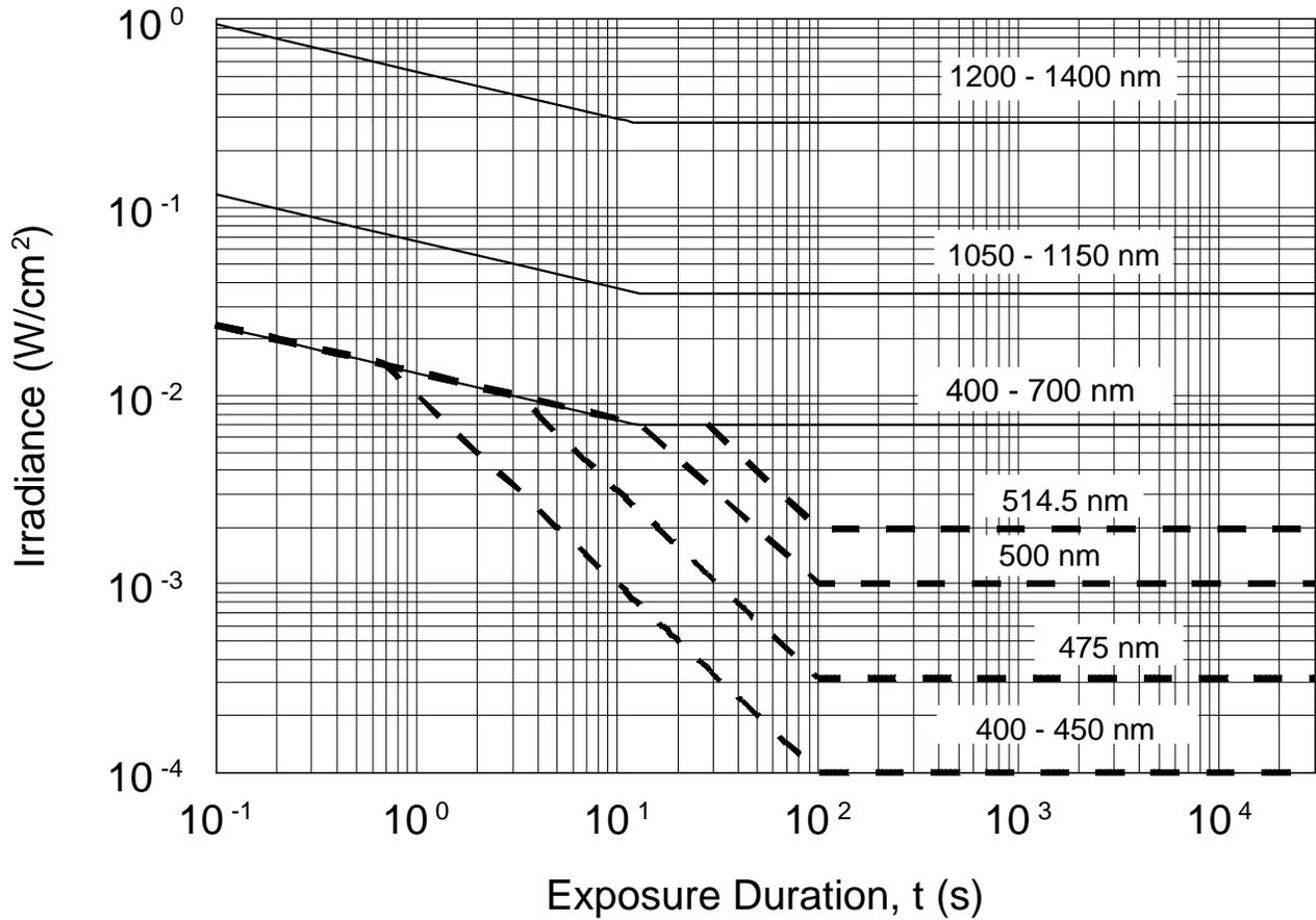
*Figure E-7. Extended source ocular maximum permissible exposures ( = 11 milliradian) for visible and near infrared (400 nanometers to 1400 nanometers) (Solid lines are maximum permissible exposures based on thermal effects, and dashed lines are maximum permissible exposures based on photochemical effects)*
