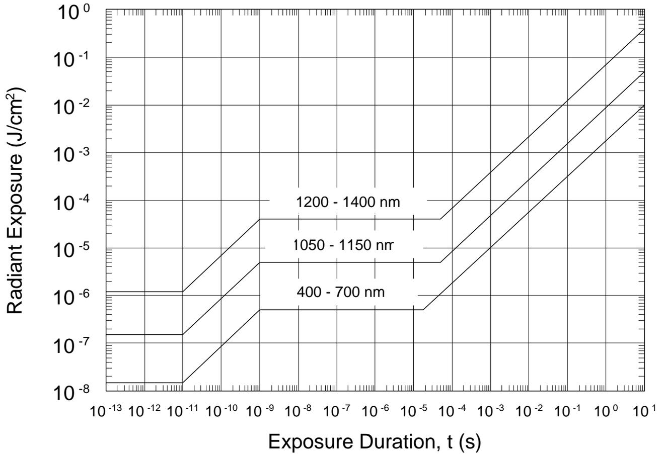
*Figure E-1. Maximum permissible exposures for visible and near infrared (400 nanometers to 1400 nanometers) for pulsed small sources*
