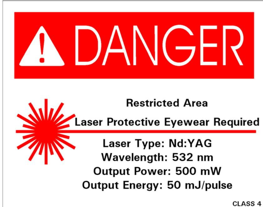
*Figure 5–3. Sample warning sign for Class 4 double neodymium:yttrium aluminum garnet laser*
